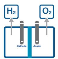
FIG. 7. A H<sub>2</sub> electrolyzer separates water into H2 and oxygen molecules using electricity.
