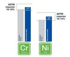
FIG. 5. High-quality components that contain higher levels of chromium and nickel will more readily resist corrosion and H<sub>2</sub> embrittlement.
