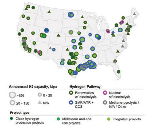
FIG. 13. Operational and active H2 production projects in the U.S. These installations/projects represent approximately 12 MMtpy of H2 production capacity.39 Source: U.S. DOE.
